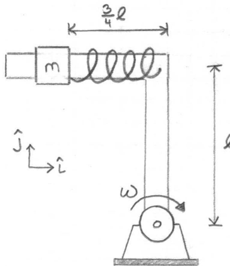
Given:  $l = 0.4 \text{ m}$ ,  $\omega = 2 \text{ rad/s}$ ,  $k = 6 \text{ N/m}$
